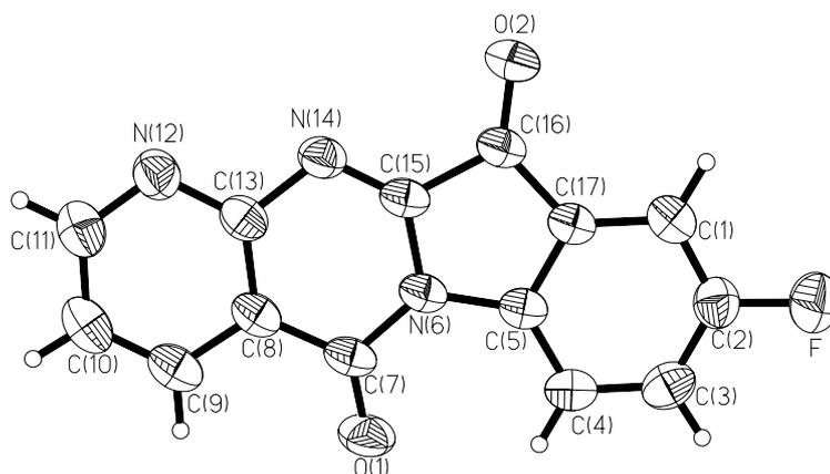
**Figure 6.** Thermal ellipsoid plot of molecule **4** showing the atom numbering used for the X-ray crystallographic report. Ellipsoids are drawn at the 50% probability level and H atoms are represented by circles of arbitrary radii.
