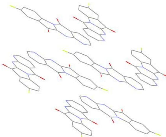
**Figure 8.** The molecules of compound **4** are arranged in layers tilted at a 7.64° angle relative to the (001) plane, with a 3.496(9) Å average intermolecular separation.
