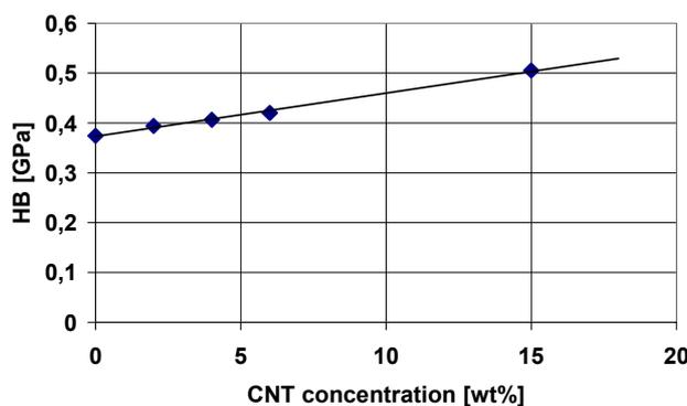
**Figure 6.** Hardness as function of MWCNT concentration in the nanocomposites.
