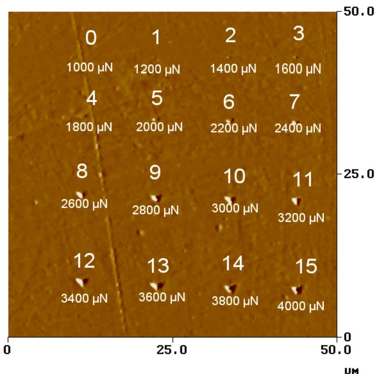
**Figure 3.** Principal schema of 4x4 array of indentations, numbers on each indentation triangle indicating order and maximum load in  $\mu\text{N}$  of the indentation.
