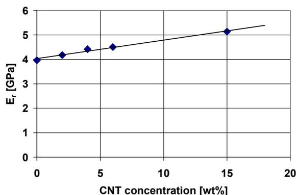
**Figure 7.** Young's modulus as function of MWCNT concentration in the nanocomposites.
