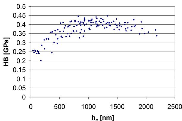
Figure 4. Hardness as function of contact depth in the sample with 2wt% MWCNT.
