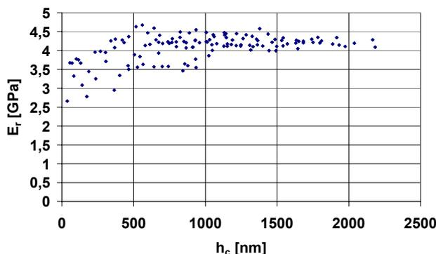
Figure 5. Young's modulus as function of contact depth in the sample with 2wt% MWCNT.
