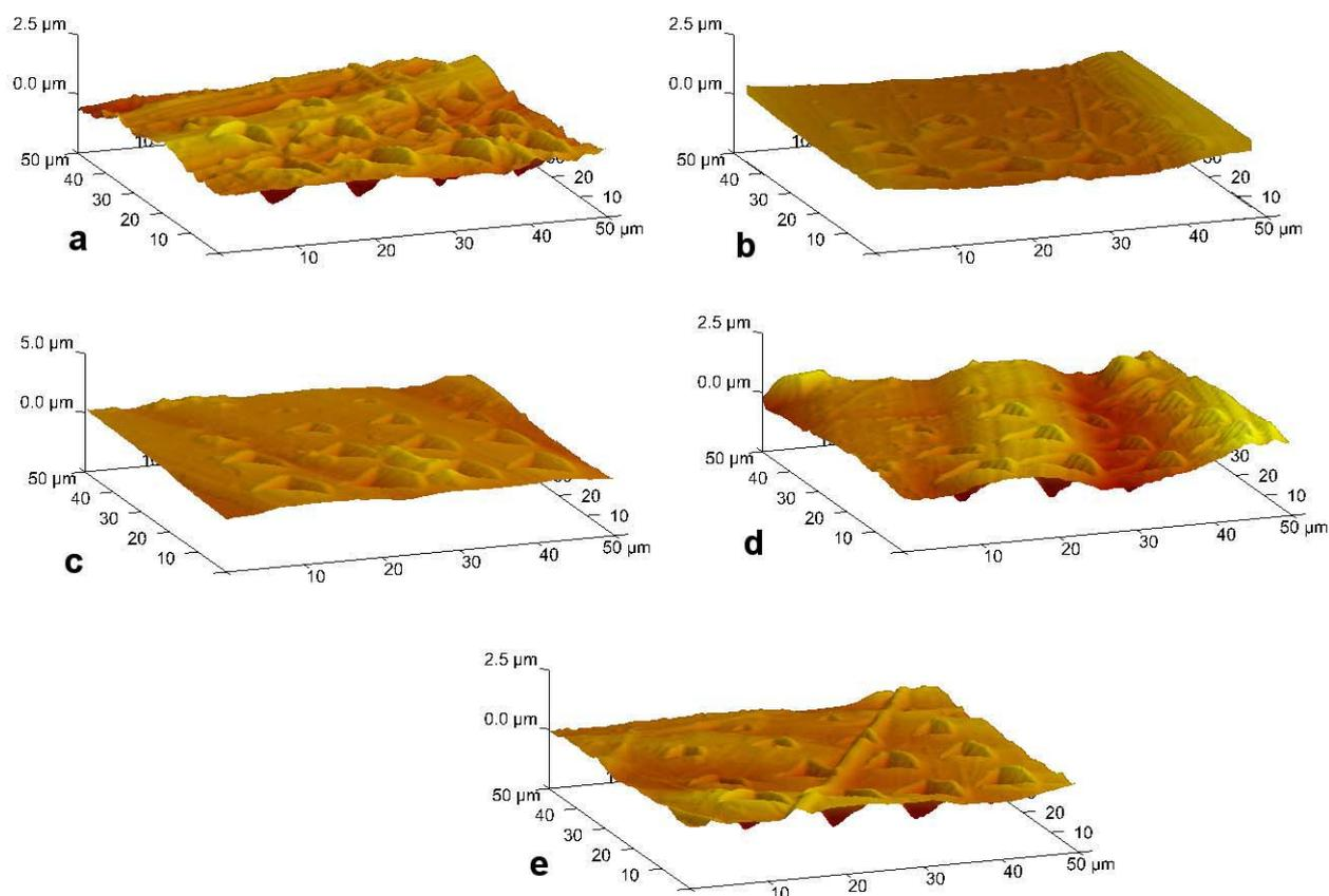
**Figure 8.** AFM images of the indented surfaces of pure PC (a), PC with 2wt% MWCNT (b), PC with 4wt% MWCNT (c), PC with 6wt% MWCNT (d), and PC with 15wt% MWCNT (e).
