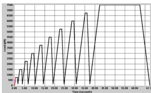
**Figure 1.** Cyclic loading program used in indentation experiments.
