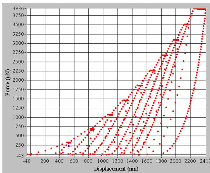
**Figure 2.** Load curve of an indentation experiment.
